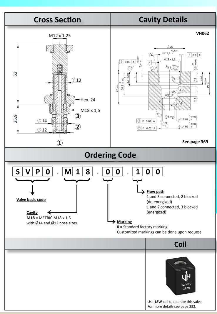
A Solenoid operated, 3 way 2 positions, spool type, direct acting, screw-in hydraulic directional cartridge valve.
